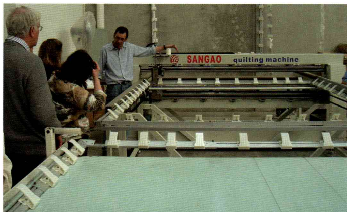
Trevor shows the MPAB group the quilting machine that stitches the cover to the fleece insert material. This machine puts 8,566 stitches on each quilt in about 5 minutes.
