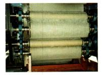
caused during the scouring process (alpaca is usually less entangled than sheep wool due to its low scale protrusion). The fibre is partially aligned (short and long fibres) and delivers what is called a carded sliver. A large amount of the burr and seed content is removed during this carding process.
