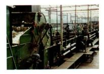
cleaning process. Here it is washed with warm water and detergents and rinsed in the final bowl. Alpaca fibre has a very low grease content.
