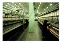
that can be used in the spinning process. This is called a roving. This process is carried out a number of times until the desired thickness of roving is obtained.
