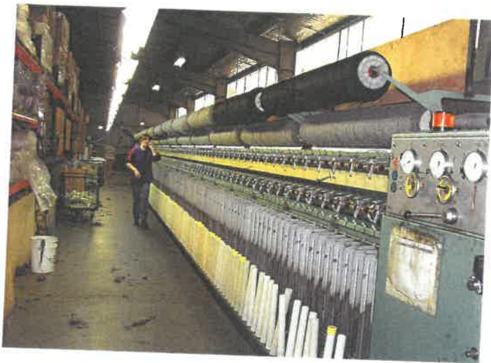
7. The carding cones are transferred to the yarn spinning machine and wound onto yarn cones.
