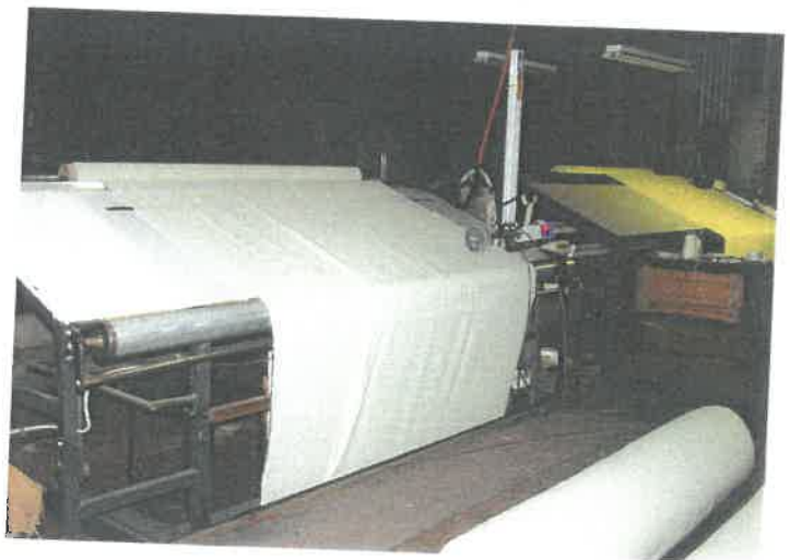
10. After weaving, this Perch rolls through the bolt of fabric and is manually checked for imperfections.
