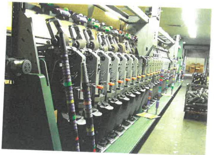
8. The yarn cones are taken to the Winder machine. The Winder checks for imperfections and uses electronic air splicing which creates an even thread.
