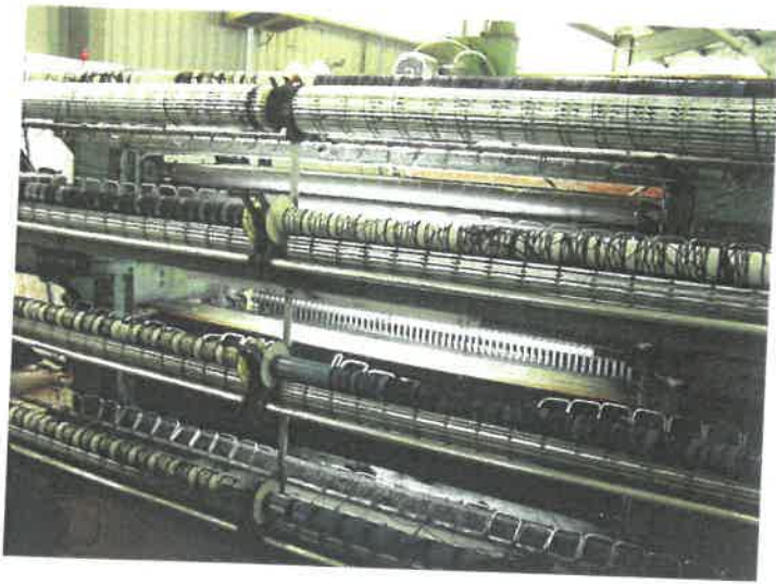
5. Loosely carded alpaca fleece is wound onto carding cones.
