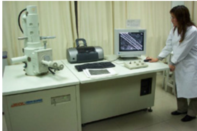
Fig. 3.5 Erdos cashmere group has been investigating the cuticle scale properties of Chinese cashmere using the scanning electron microscope.
