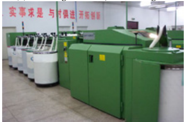
(f) Producing cashmere slubs for woollen spinning, Erdos, Inner Mongolia
