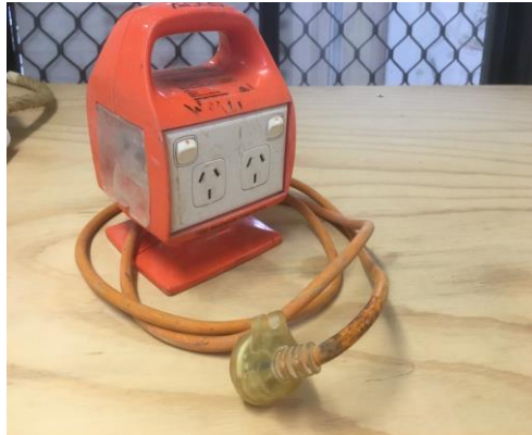
RCD mounted in box
