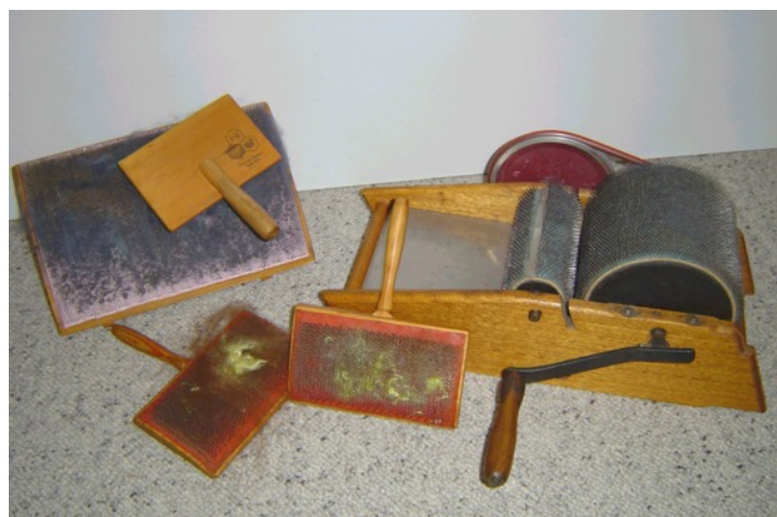
Examples of carding equipment available to the crafts person. Left to Right: Board Carder, Hand Carders and Drum Carder.
