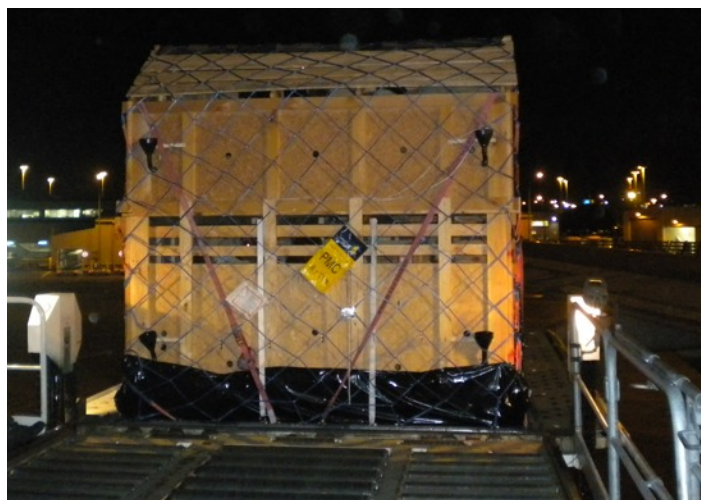
Crate being loaded onto aircraft in Auckland, 4 black funnels for refilling the water troughs during flight are clearly visible
