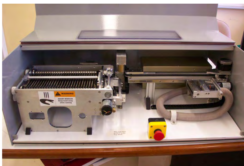
Figure 5.7. The laboratory fibre measurement instrument the OFDA4000.
